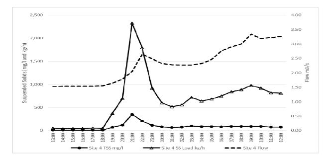
Figure 2: Example graph showing suspended solids concentration (mg/l) and load (kg/h) with flow (m<sup>3</sup>/h) in the main By Brook during wet weather event 1
